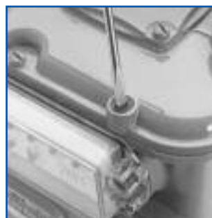
Screwdriver blade must break security seal to remove cover.
